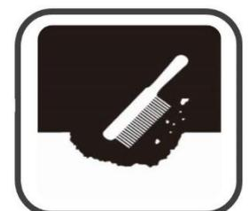
**Fill** the hole with PHF Cold Mix (make middle slightly higher than the sides - this is called crowning - depending on the size of the repair give yourself a 5-10mm crown - this counteracts the subsidence caused by compacting
