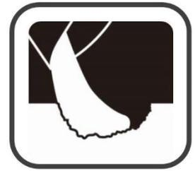
Compact a compactor is recommended for larger holes or timber post for ramming can be used on smaller holes very effectively
