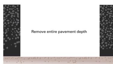
Full depth repair completed in 100mm layers
