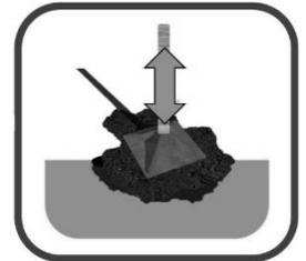
Driving back and forth over the crowned PHF Cold Mix in a vehicle will provide sufficient compaction in most pot holes
