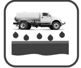
Apply RDC at 2ltrs per sqm, ensuring uniform coverage of all material to be treated and avoiding run off by allowing the product to soak in and apply in multiple applications.
