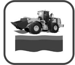
Take pre-blended aggregate to site and spread at designed depth, uniformly.
