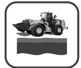
The loader is to approach the stock pile from all directions lifting the product and aggregate up to a 1.5mtr head above the stock pile and dump it over the leading edge of the pile. This process is to be repeated until the product is uniformly mixed.
