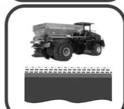
The stabilizing agent (dry powder) shall be uniformly spread at the specified application rate across the pavement
