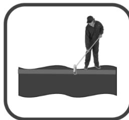
When applying FCM Co-Polymer, apply 50% of the FCM Co-Polymer at Initial Step 6G and then apply the remaining 50% in the process of point 7 slurrying.
